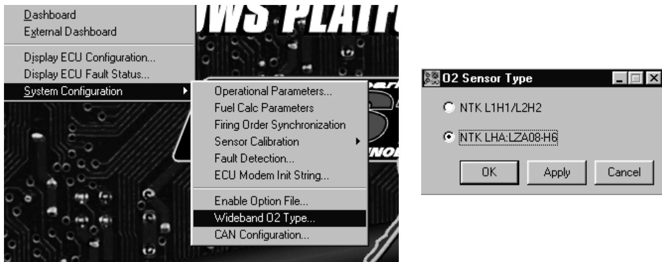
**NOTE:** An incorrect “O<sub>2</sub> Sensor Type” setting can cause erroneous O<sub>2</sub> readings. If tuning is performed or closed loop fuel corrections are made based on erroneous O<sub>2</sub> readings, the engine may run richer or leaner than intended and engine damage could result.
